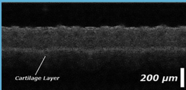
Spectral-domain OCT cross-sectional image of a mouse ear. The image provides both the tissue's topographic surface information and underlying microstructure, showing the cartilage layer within the ear.
