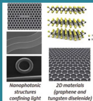
Nanophotonic structures (photonic crystal cavity, ring resonator or waveguide) coupled with two dimensional materials constitute a scalable platform for strong light-matter interaction. Such a platform is critical for engineering low-power opto-electronic devices.
