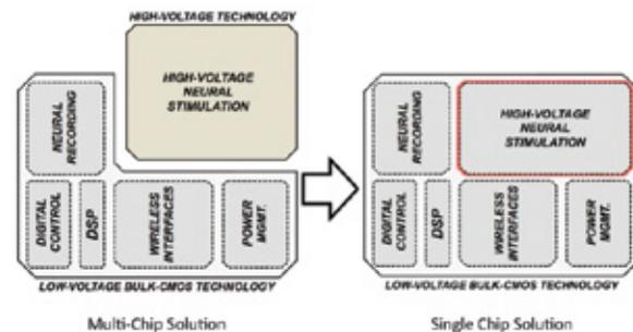
By developing high-voltage compatible circuits in a low-voltage CMOS process, all blocks of the system are placed onto a single chip, realizing drastic improvements to form factor and cost.
