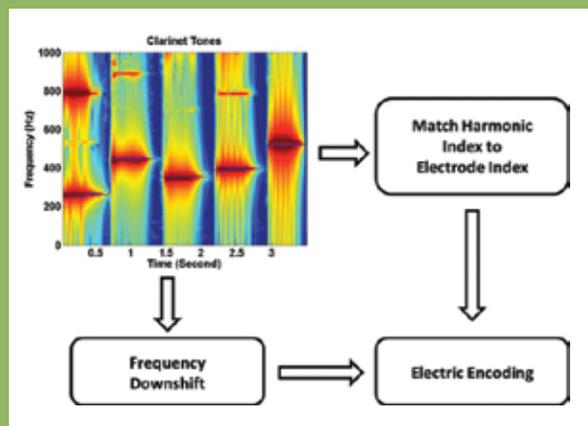
An example of the estimated clarinet music pitch (thin blue line in top left) and block diagram of HSSE processing for cochlear implants.
