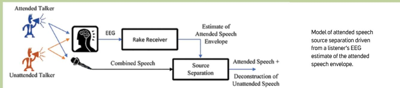
In many modern digital communication systems, specifically technology used in cell phones, background noise is successfully minimized by implementing a technique known as a “rake receiver.” This type of radio receiver utilizes the multiple paths a signal takes from the transmitter to the receiver by “raking” the multi-path signals into a single coherent signal, effectively improving the quality of what is received.
