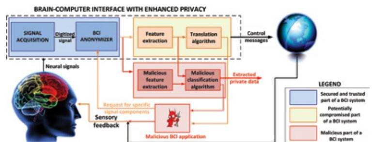
A block diagram of a BCI with the proposed "BCI Anonymizer." Malicious components (blocks "malicious feature extraction," "malicious classification algorithm" and "malicious BCI application") may request data, but will not receive a response from the "BCI Anonymizer."
