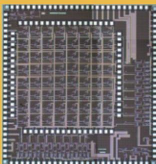
A front-end chip was designed utilizing row-column architecture.
