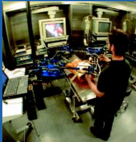
The Blue Dragon, a device for measuring the properties of endoscopic tools and for objectively evaluating a surgeon's performance.
