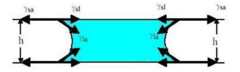
Figure 2: "Model One" of Capillary Forces
